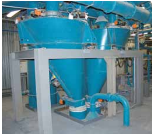
EIRICH RV19 intensive mixer Sand and binding agent scale Movable scale and volumetric hopper
