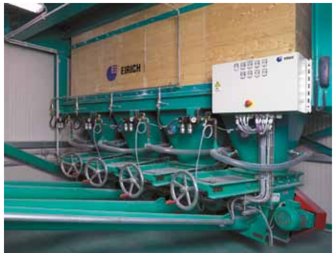
EIRICH R15 intensive mixer Additive storage and feeding Single-spout packer with manual palletizer
