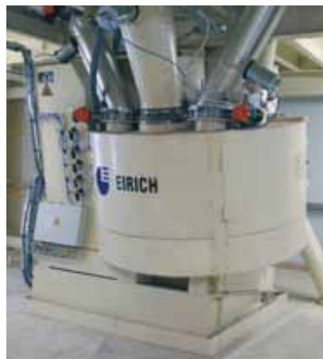
EIRICH RV19 intensive mixer with a 10° tilt
