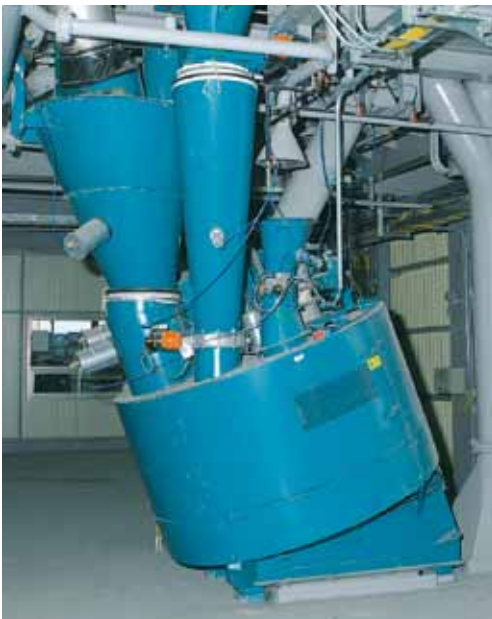
EIRICH R19 intensive mixer Swap containers above the movable additive scale Main component scale with volumetric hopper Movable scale
