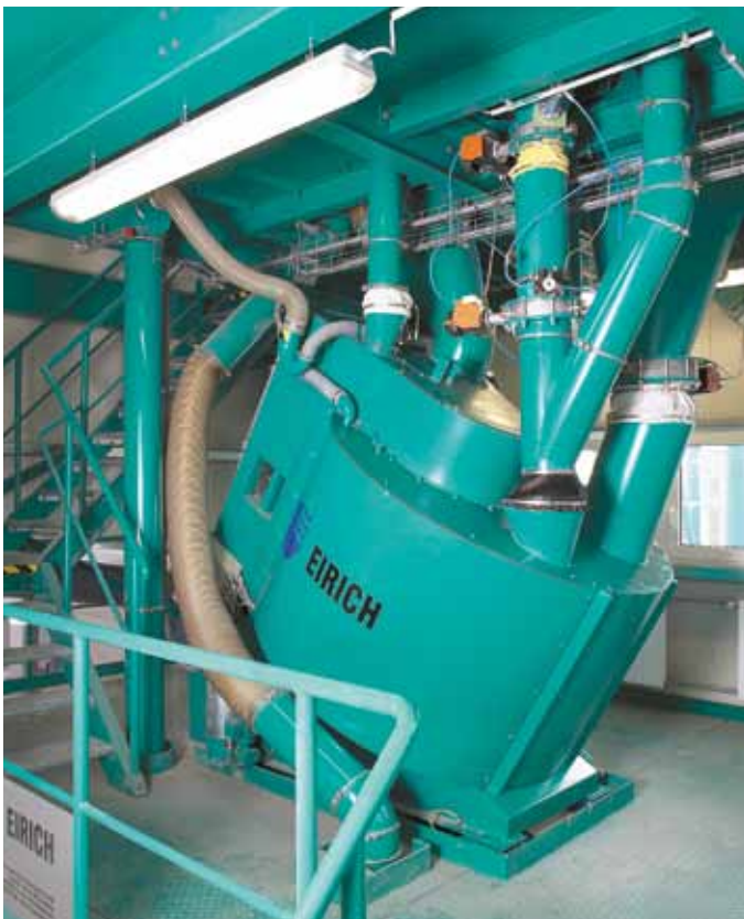
EIRICH R15 intensive mixer Additive storage and feeding Single-spout packer with manual palletizer
