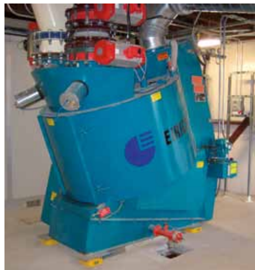
Pneumatic conveying system EIRICH RV15 intensive mixer with a 10° tilt Raw material batching
