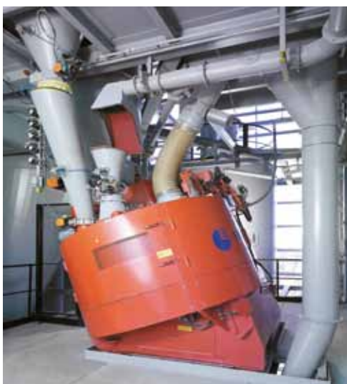
Factory building Vertical lift above the mixer EIRICH RV19 intensive mixer Finished product discharger with bagging station
